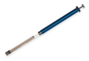
The 800 series syringes are the reinforced plunger version of the original 700 series syringes. Attached to the flange of the syringe is a blue Syringe Holder. The Syringe Holder provides a spot to hold the syringe that will not heat up the barrel causing dispense inaccuracies.
