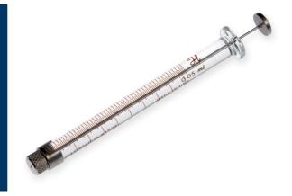
The 1700 series syringes are the gas tight version of the original 700 series syringes. This series of gas tight syringes is ideal for dispensing volumes from 1  $\mu$ L up to 500  $\mu$ L. A variety of different terminations and needle options are available in this series.
