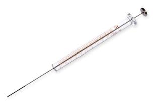
The needles on Thin Layer Chromatography (TLC) syringes are coated from the point for 3/4" with a PTFE-coating. The coating reduces the surface tension between the needle and the liquid making it ideal for reproducible sample spotting.
