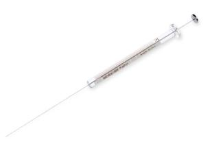
On-column injection employs the direct introduction of the liquid sample into the column. This is very useful for the analysis of thermally unstable samples and avoids boiling point discrimination.
