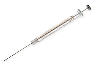
The needles on Thin Layer Chromatography (TLC) syringes are coated from the point for 3/4" with a PTFE-coating. The coating reduces the surface tension between the needle and the liquid making it ideal for reproducible sample spotting.
