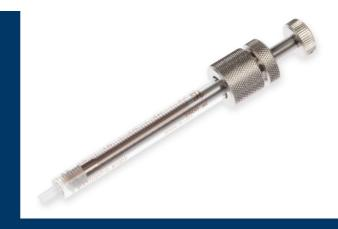
Threaded Plunger Syringes are for applications requiring extremely precise plunger movement or minute fluid manipulation. You can dispense from 0.33 to 37.79 µL per plunger revolution depending on the syringe volume.
