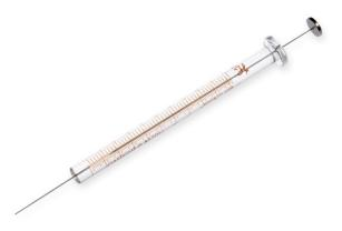
Gel Loading Syringes are designed with small gauge needles that are perfect for loading the lanes on an electrophoresis gel. The most common application is for multiplex DNA sequencing methodologies.
