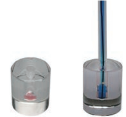
Measuring 15 µL sample with the micro container
