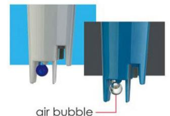
The inner solutions in pH electrode's glass bulbs are usually in liquid form, which could generate air bubbles from time to time when using. If not removed properly, the air bubblett could cause meter's malfunctioning. The 60-Z series pH electrodes adopt a unique blue gel inner solution, which would not flow and never generates air bubbles. The meter can function well even when being placed upside down.
