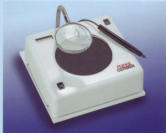
ColonyStar with clear glass plate and dark illumination area (see accessories). Indirect illumination (sideways) for bright culture-media (e.g. Reference-determination of the total amount of colonies with Plate Count Agar)
